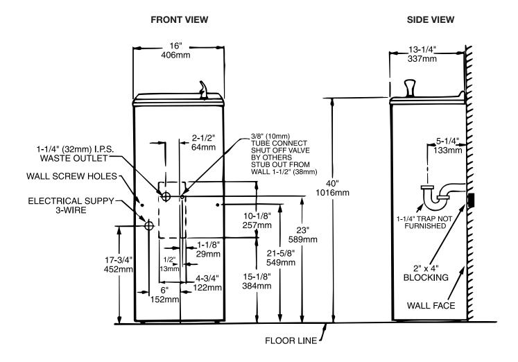
NOTE: Minimum wall clearance for air flow is 4 inches (102mm) on either side. NOTE: A service supply stop must be installed at the cooler inlet line.
